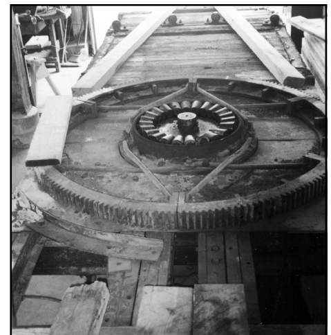
D&RGW Pile Driver OB main gear and bearings. – Photo © Tom Simco.
